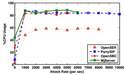
Fig. 7. Average CPU usage vs. Attack Rate
