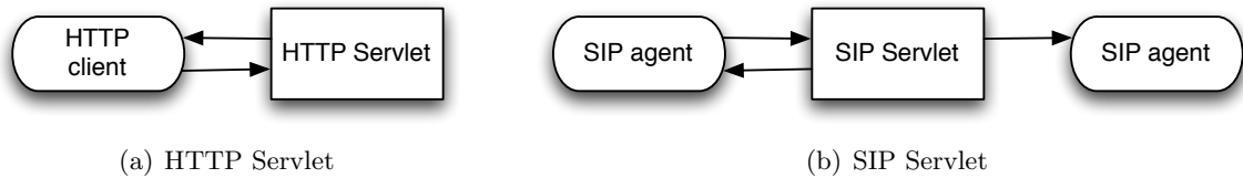
Figure 4.5: SIP servlets handle a peer-to-peer protocol while HTTP servlets handle a client server protocol.
