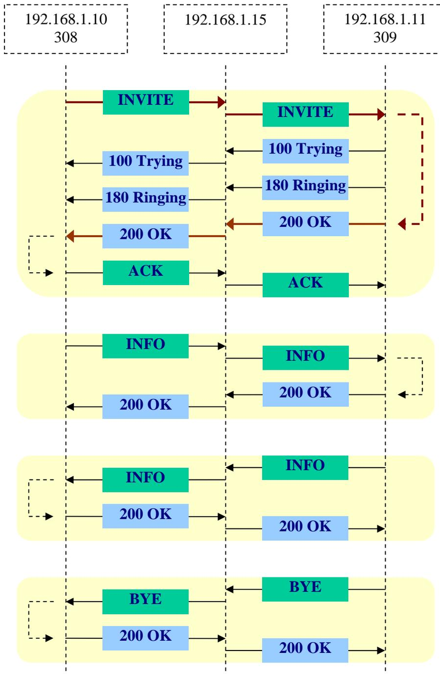
During the phone conversation there are two transactions with INFO messages. These transactions correspond to transmission of DTMF signals via SIP messages. The first INFO message tells that the digit “2” is pressed on the calling phone for 4800 milliseconds. The second INFO message tells that the digit “3” is pressed on the callee phone for 480 milliseconds. To make sure that SIP INFO messages are transmitted, we must specify in SIP phones the transmission of DTMF signals with SIP messages:
