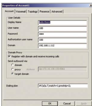
Figure 7. Configuration of X-Lite for direct calls
