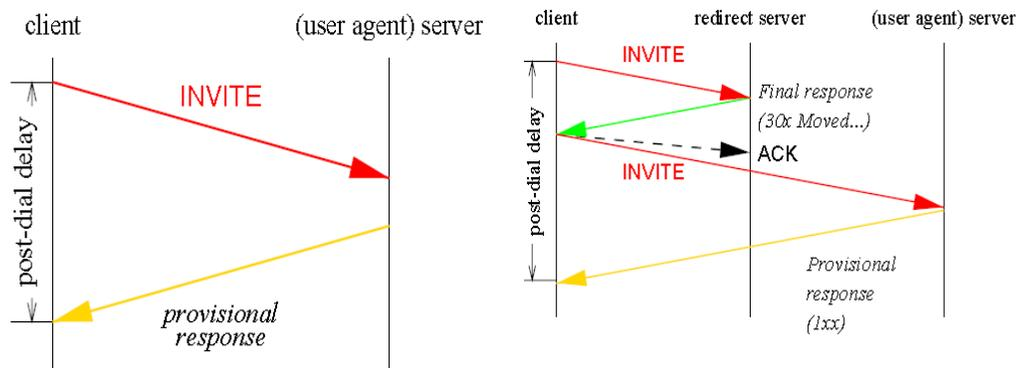
Figure 3. Call setup between SIP client-server
