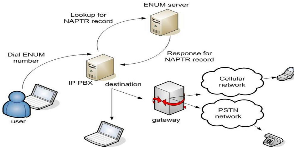
Figure 2. Flow Communication via ENUM
