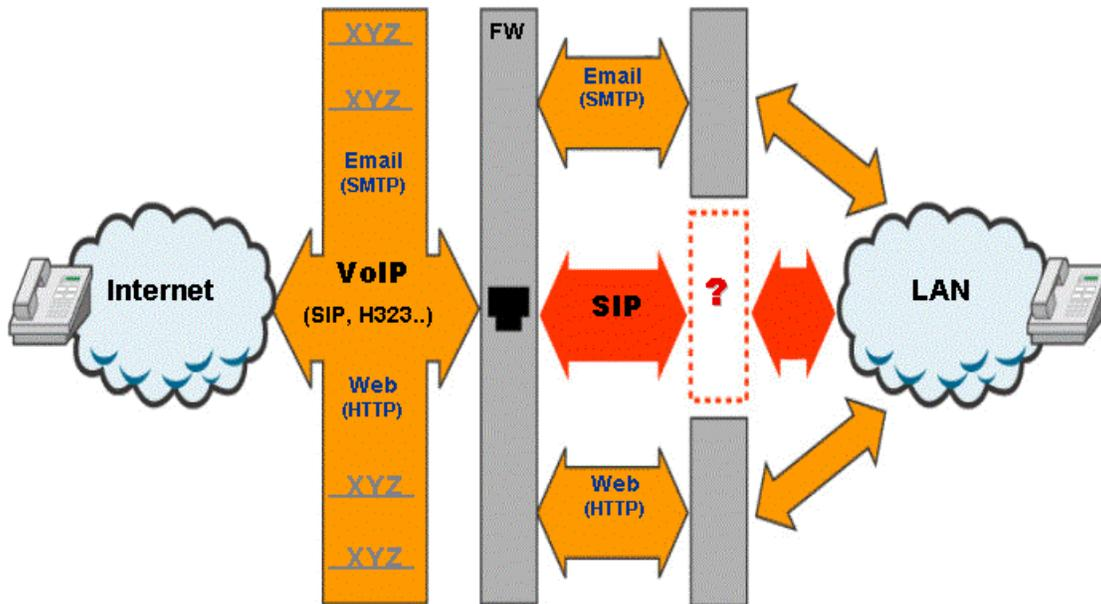
NAT is commonly used to preserve IP addresses. For SIP to function through a firewall, the NAT must be SIP-aware, in order to modify SIP messages and to control the opening and closing of UDP ports used for media. In the future, if signaling encryption becomes commonly used, in order to function, the NAT must be able to decrypt/re-encrypt the SIP messages.
