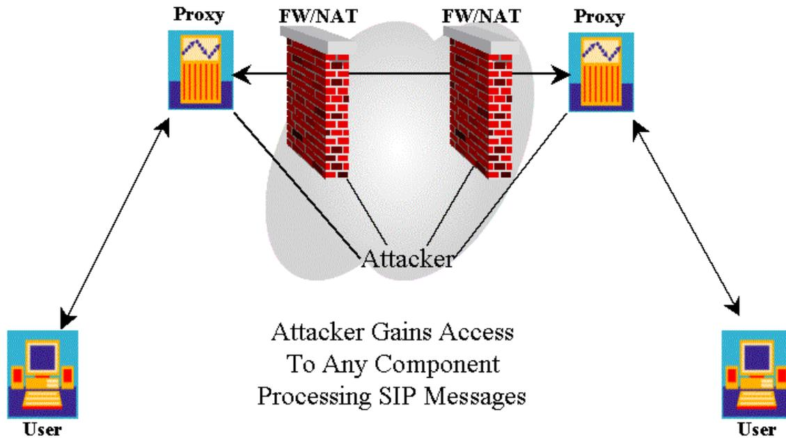
SIP messages have no built-in means to insure integrity. By manipulating SIP messages, an attacker can execute the same types of attacks described for registration hijacking and proxy impersonation.
