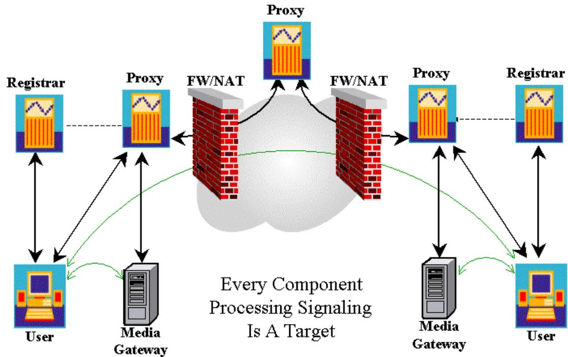
DoS can take the form of malformed packets, manipulating SIP states, and simple flooding, such as a “REGISTER” or “INVITE” storm (a flood of packets). Research has shown that many SIP implementations are highly vulnerable to these types of attacks. For examples, see the following link:
