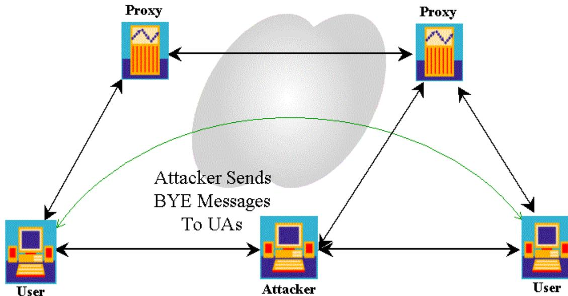
If a UA does not check the available packet values, the attacker may not even need to observe the call signaling. If the attacker knows the address of a continually active UA (such as your media gateway, AA, IVR, trading floor phone, etc.), they can send BYE messages, causing the call(s) to be torn down. Another example of message tear down is flooding the firewall with BYE messages, possibly tearing down UDP ports opened for legitimate calls.
