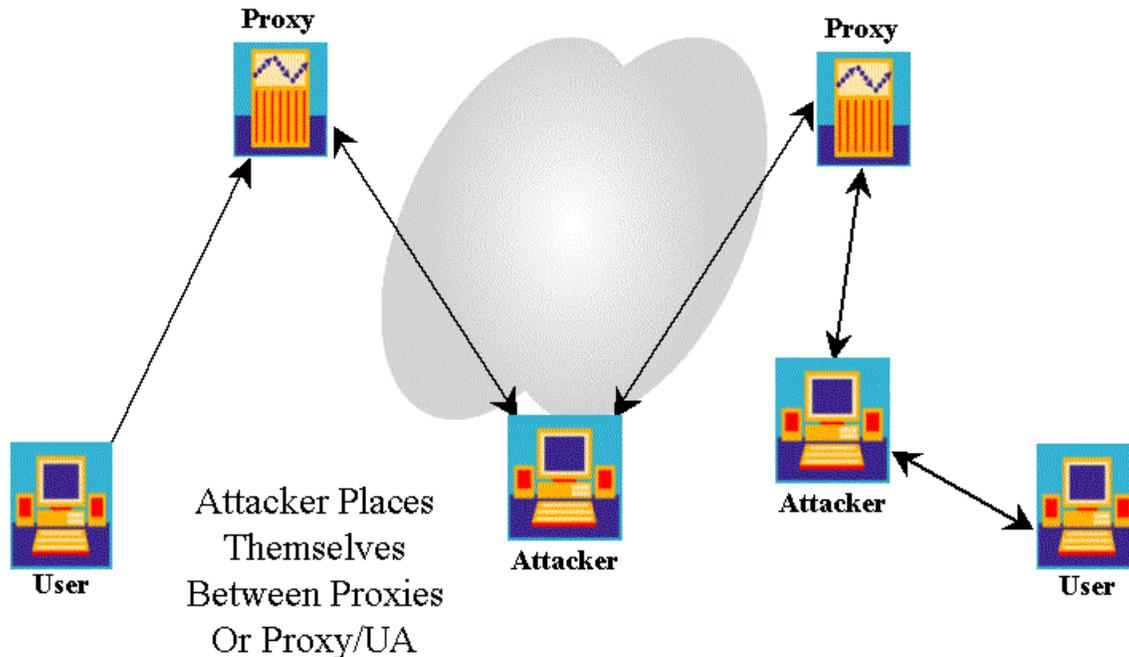
Your UAs and proxies normally communicate using UDP and do not require strong authentication to communicate with another proxy. A rogue proxy can therefore insert itself into the signaling stream through several means, including Domain Name Service (DNS) spoofing, Address Resolution Protocol (ARP) cache spoofing, and simply changing the proxy address for a SIP phone. An impersonated proxy has full control over calls and can execute the same types of attacks described for registration hijacking.
