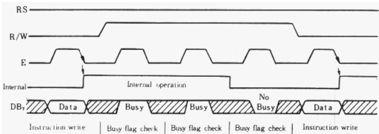
The above picture does one write followed by one read. To do this, data must be presented on the 8 data pins and then the enable line is pulsed. To perform a read, change the R/W line to 1 and wait until the busy signal on DB7 goes to 0, then the data will be presented on the next pulse.
