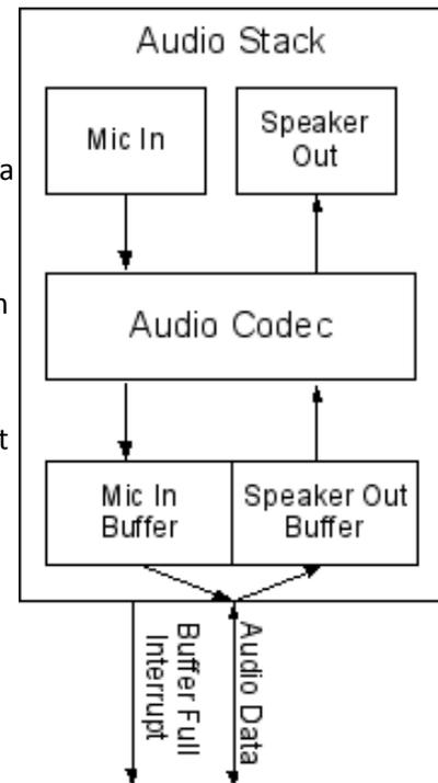
**The audio stack, consisting of the physical devices, codec, memory, data and interrupt lines.**
