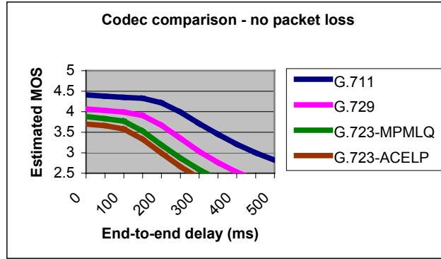
Figure 9. If there were no jitter and no packet loss, the MOS would be influenced only by the end-to-end delay and choice of VoIP codec. This graph shows the effect on the MOS of just end-to-end delay for four example codecs.
